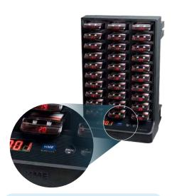
Auto-numbering of your IQ pagers: Press "prog" for 10 seconds until the beep, release the button en press again for 2 seconds until the beep.
